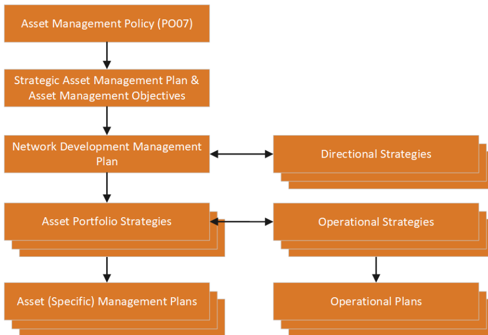
FIGURE 1 ASSET MANAGEMENT SYSTEM DOCUMENT HIERARCHY (UNDER DEVELOPMENT). NETWORK RELIABILITY STRATEGY IS CLASSIFIED AS AN OPERATIONAL STRATEGY.
