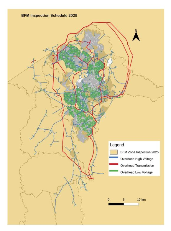
This is the flying zone (Bushfire Management Zone comprising of BAZ and Rural Land). Evoenergy use LIDAR-enabled Aircraft to fly multiple sections of power lines capturing data on vegetation, conductors, poles and other structures. Further information is available on the <a href="Evoenergy website">Evoenergy website</a>.
